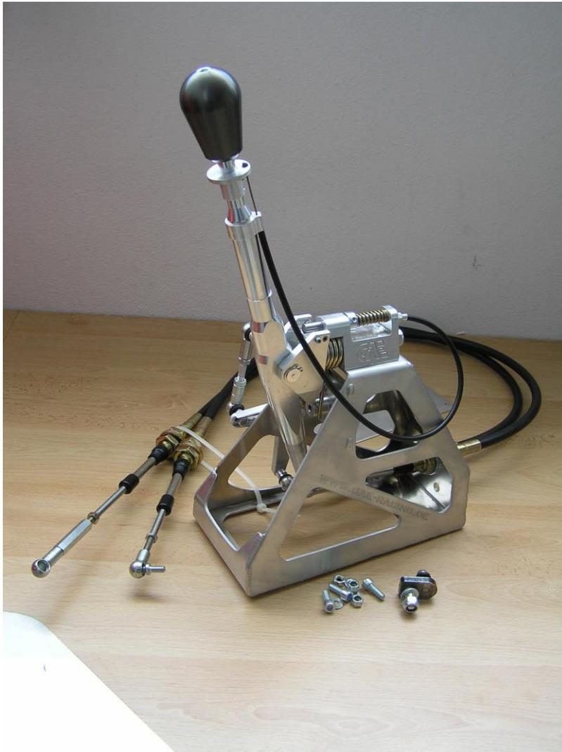
The shifter is intended for Racing Cars without interior equipment. If center console is mounted, it must be dismantled or modified to achieve an acceptable space for the cables.
