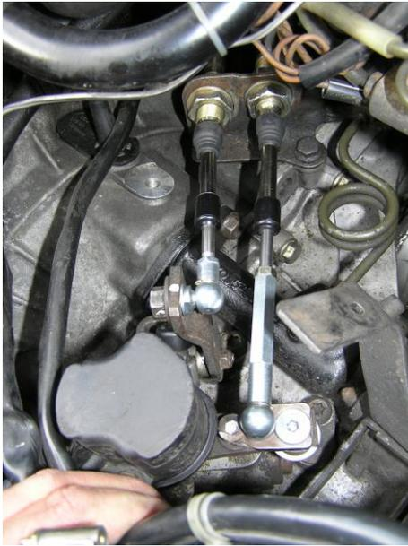
Remove the original parts of the shifter including the shifting cable
