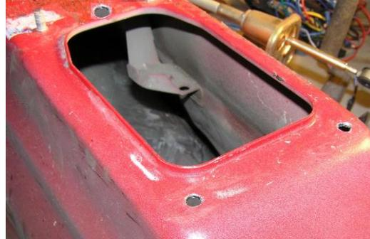
Before drilling you must check if the cables have enough space Engineroom. If not, change position of holes as far as necessary.
