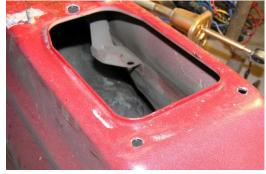
Before drilling you must check if the cables have enough space Engineroom. If not, change position of holes as far as necessary.
