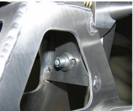
Now adjust the middle position of the gearshift by adjusting the lower spring stop under the unit with Allen wrench 5mm.
