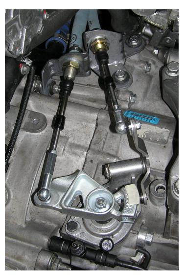
Ensure the space of the cables to the Exhaust, if necessary mount additional clamps and heatshields
