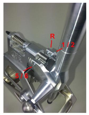
Remount the connection rod now Adjust it fitting to the both balls
