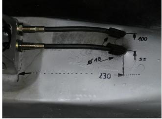
The measurements refer to the outer edge of the mounted shifter; there for you mount the shifter with one screw and line it up.
