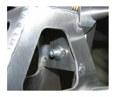
Secure the seats on the cables in the selector-tower. Select level 1 / 2 with gearshift and adjust the fitting stop screw until the gears 1
