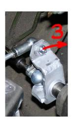
In middle position the gearshift should be slightly turned to the right.
