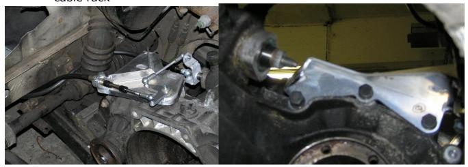
Mount connecting Rod "S" on the gear unit entry lever (Picture shows the old Version) Mount both of the cables at the unit. The choose cable to the L-Lever left has to stand out as much as possible of the case, inside there is no threads to see.
