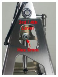
Now adjust the wanted middle position of the gearshift and adjust the lower spring stop under the unit with allen
