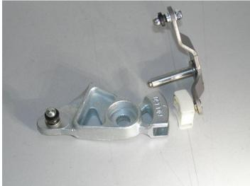
Drill out the stock bolts (8mm) on both levers and mount the delivered Ball pins:
