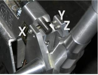
Now select gear 5 / 6 by the gearlever and turn stop screw X
