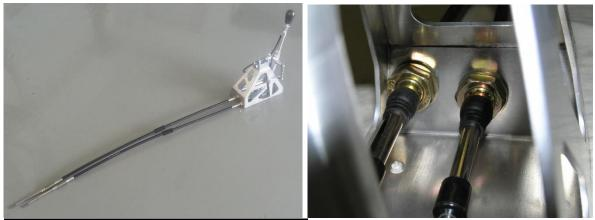
Remount all on parts on the outside of the cables S & W. The longer shift cable (S) have to be mounted to the middle hole of the shift tower. Accordingly, the shorter cable (W) left side (to L-Lever) The cable must stand out as far as possible from the shift unit, inside is not thread visible:
