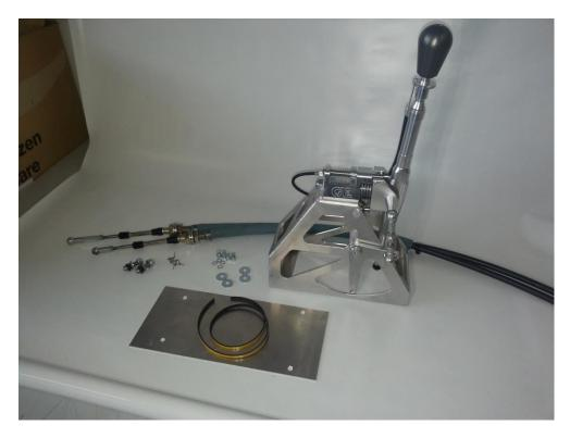
The shifter is intended for racing cars without interior equipment. If center console is mounted, it must be dismounted or modified to achieve an acceptable space for the cables. The new unit should be mounted directly on to the floorboard, so part of
