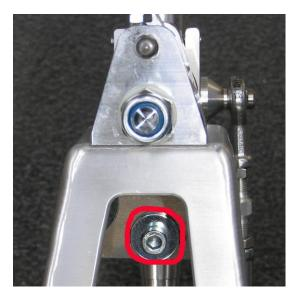
Adjust the Spring stop under the Shift unit: The Shiftlever hat to stand slightly to the left side (about 3-5 deg)
