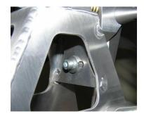
• Push the connector rod back to ball pins on the left side of the shift unit and adjust the connector rod (right/left spindle) for pushing on without moving the lever.
