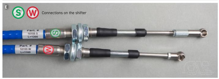
The shifter is intended for racing vehicles without interior equipment. If the center console is installed, it must be removed or cut out to the extent that a corresponding clearance for the shift cables is ensured. The gearshift bracket should be screwed directly onto the sheet metal of the center tunnel, any existing carpet must be cut out.
