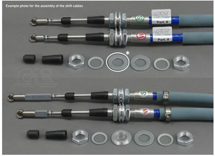
$^{\star}$  With the underfloor shifter, this washer is omitted inside the shifter box!
