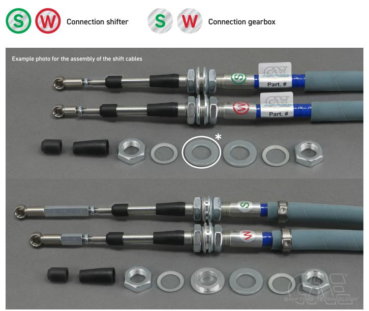
$^{m{*}}$  With the underfloor shifter, this washer is omitted inside the shifter box!
