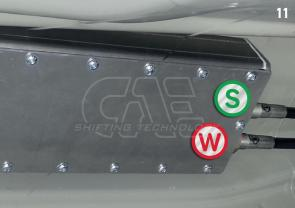
When installing, immediately route the cables in the direction of the engine compartment above the gear unit. Secure the M16 nuts with the toothed lock washers supplied, do not glue them in!
