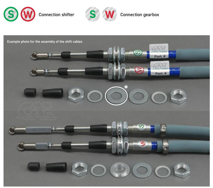
st With the underfloor shifter, this washer is omitted inside the shifter box!
