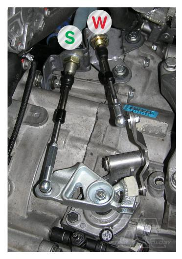
(i) PLEASE NOTE: ! Check cables for "end position free travel". When a gear is engaged, there must still be a residual travel available on the rope! (Picture A, B, C)
