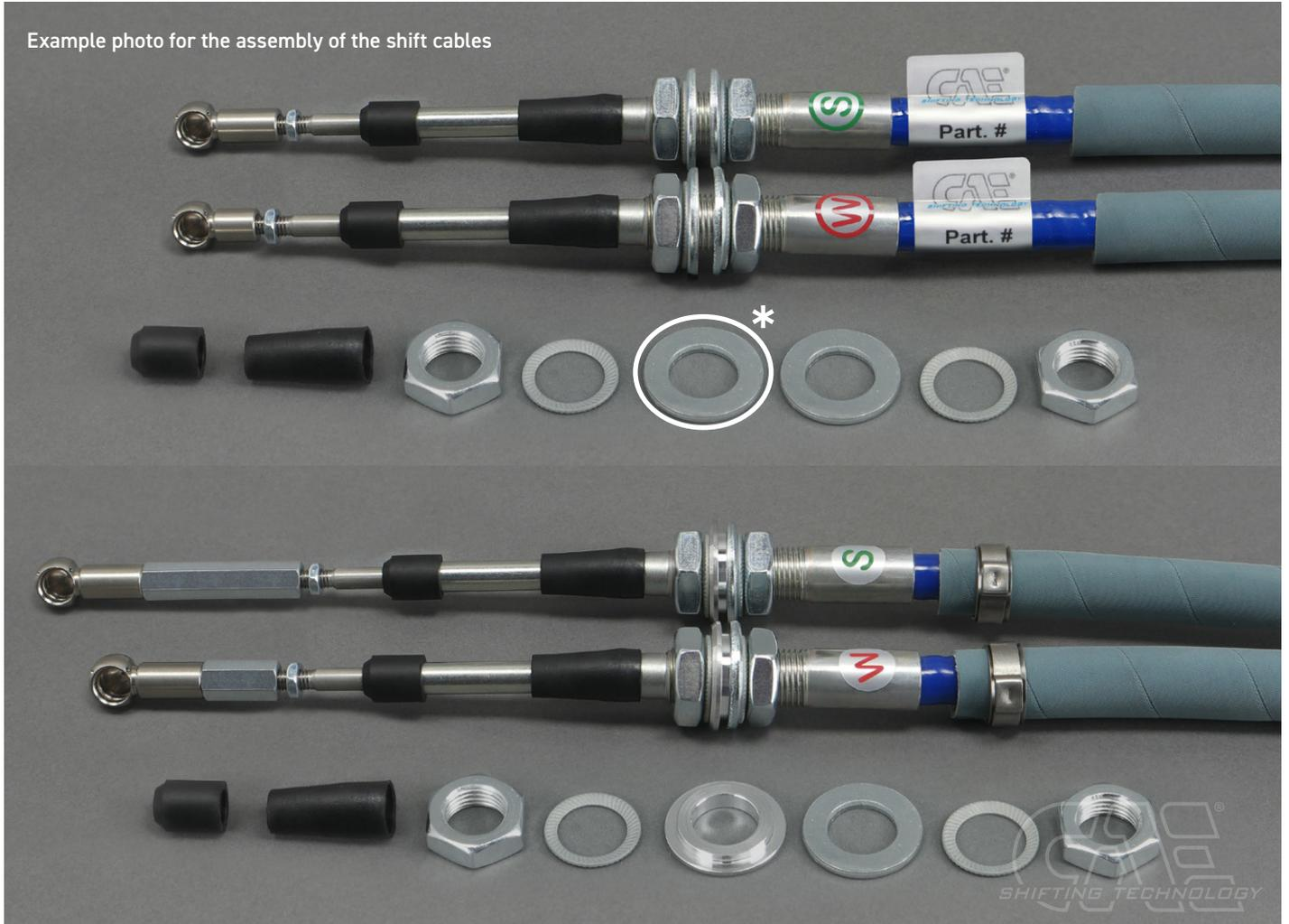
\* With the underfloor shifter, this washer is omitted inside the shifter box!
