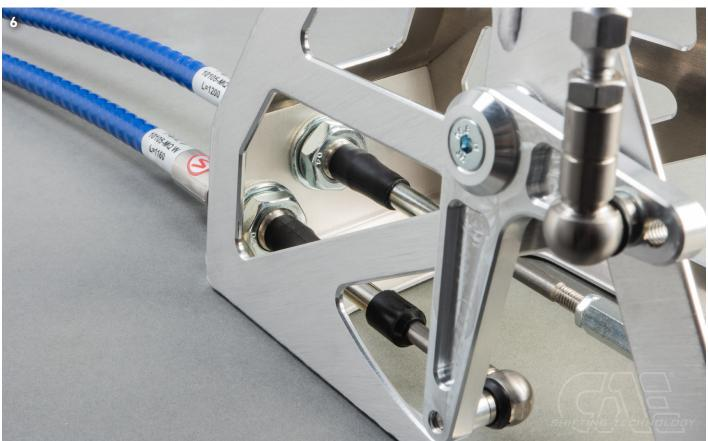
▶ Dismantle all attachments on the gearbox side of the S & W shift cables. Attach the longer cable ⑤ to the center of the shifter, correspondingly the shorter selector cable to the left. ℳ Mount the aluminum centering disk on the shift cable according to the housing bore. The shift cables must protrude as far as possible from the shift tower, no thread is visible inside the shifter housing. (Picture 6, 7)
