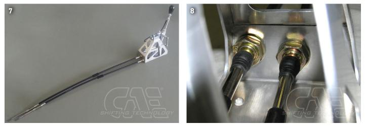
Dismantle all attachments on the transmission side of the S & W shift cables. The longer cable (s) is attached to the center of the shifter, correspondingly the shorter selector cable (w) on the left. The shift cables must protrude as far as possible from the shift tower, no thread is visible inside the shifter housing. (Fig. 8)
