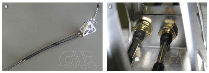
Dismantle all attachments on the transmission side of the S & W shift cables. The longer cable (s) is attached to the center of the shifter, correspondingly the shorter selector cable (w) on the left. The shift cables must protrude as far as possible from the shift tower, no thread is visible inside the shifter housing. (Picture 6)
