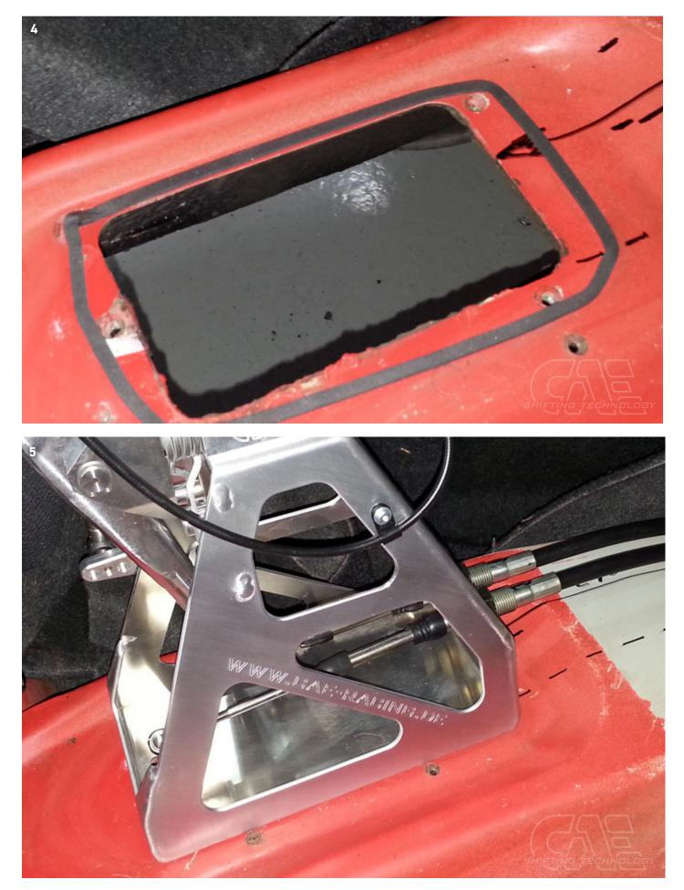
The original hole in the frame triangle of the bulkhead can be used to feed through the shift cables; this must be extended accordingly: (Picture 6, 7, 8, 9)
