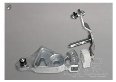
Before screwing on the switch tower, glue the enclosed foam rubber strips to the tunnel so that they seal the tunnel opening later. (Picture 4)
