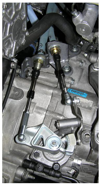
(i) PLEASE NOTE: ! Check cables for "end position free travel". When a gear is engaged, there must still be a residual travel available on the rope! (Picture A, B, C)
