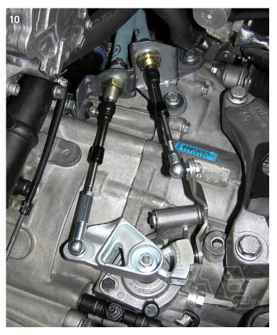
(i) PLEASE NOTE: ! Check cables for "end position free travel". When a gear is engaged, there must still be a residual travel available on the rope! (Picture A, B, C)
