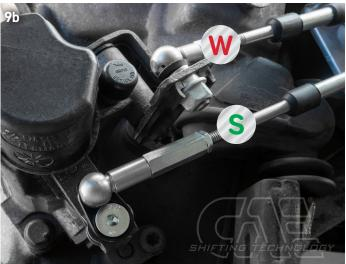
(i) PLEASE NOTE: ! Check cables for "end position free travel". When a gear is engaged, there must still be a residual travel available on the rope! (Picture A, B, C)
