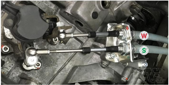
(i) PLEASE NOTE: ! Check cables for "end position free travel". When a gear is engaged, there must still be a residual travel available on the rope! (Picture A, B, C)
