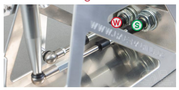
The position of the shift knob can be varied using the hexagonal extensions supplied. Always make sure that the lever does not touch anything in the end position. The following applies: The longer the pan/hexagon, the further the knob moves forward. (Bild 8) This change can be made later at any time; no further adjustment is necessary.
