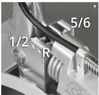
**PLEASE NOTE:** In gears 1/2 and 5/6 the grub screw must not touch the locking pin when the gear is engaged!
