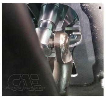
**TEST:** With 3rd and 4th gear engaged, the lateral play at the shift lever must be equal. If this is not the case, the spring stop must be re-adjusted. (0.5 mm is already a lot here)
