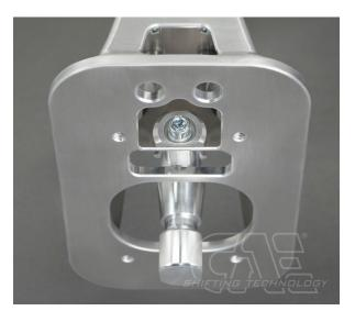
(i) The shifter is intended for racing vehicles without interior equipment. If the center console is installed, it must be removed or cut out until there is sufficient clearance for the shifter. The shifter must be screwed onto the sheet metal of the center tunnel and any existing carpet must be cut out.
