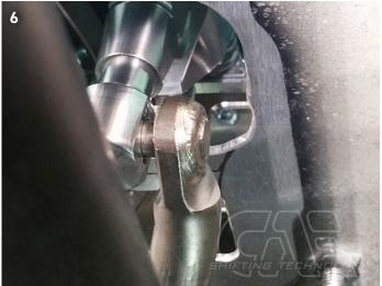
CHECK: When 3rd and 4th gear are engaged, the lateral clearance on the shift lever must be the same. If this is not the case, the spring stop must be readjusted. (0.5 mm is already a lot here).
