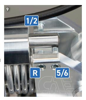
After complete assembly of the shifter, lubricate all moving parts, we recommend Würth HHS 2000. Glue in all nuts / screws during assembly!
