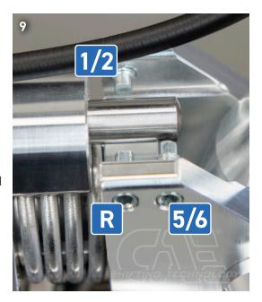
i After complete assembly of the shifter, lubricate all moving parts, we recommend Würth HHS 2000. Glue in all nuts / screws during assembly!
