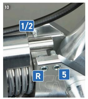
(i) After complete assembly of the shifter, lubricate all moving parts, we recommend Würth HHS 2000 (does not apply to plastic pans) Glue in all nuts / screws during assembly! Never kink shift cables!
