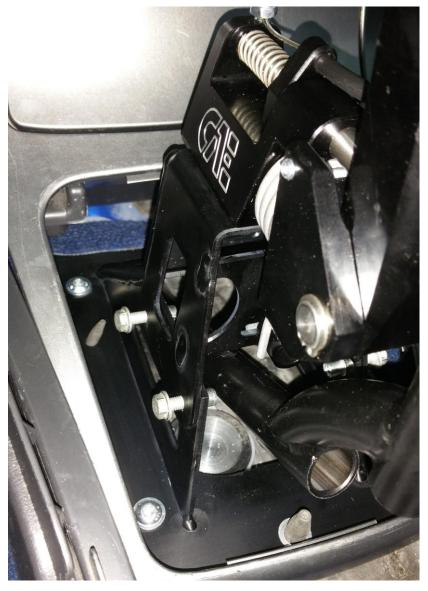
grease the main bolt ot the shift rod
