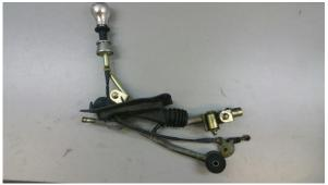
Hit the double split pin out of the rod connector to the upper side and remove the reverse gear attachement. Then loosen the backwards bracket and remove the complete shift unit to the upper side.
