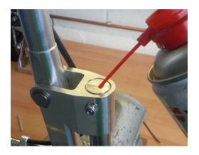
!!!Grease the Main bolt and the hole for it good before assambling !!! Take care that the bolt and hole is not damaged !!!
