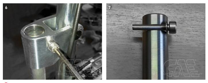
(i) Regularly spray penetrating oil into the collar at the tip of the pilot bolt. This is absolutely necessary for proper functioning. Remove excess grease and keep surfaces clean.
