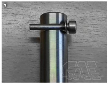
(i) Regularly spray creeping oil into the collar at the tip of the pilot pin. This is absolutely necessary for proper functioning. Remove excess grease and keep surfaces clean.
