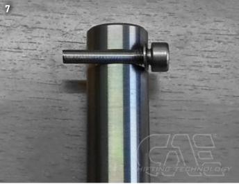
Regularly spray creeping oil into the collar at the tip of the pilot pin. This is absolutely necessary for proper functioning. Remove excess grease and keep surfaces clean.
