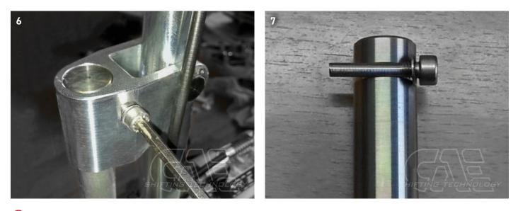
(i) Regularly spray creeping oil into the collar at the tip of the pilot pin. This is absolutely necessary for proper functioning. Remove excess grease and keep surfaces clean. NEVER spray cleaner or degreaser into the connection. This applies to all bearing points of the shifter.
