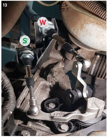
▶ Fasten the cables to the gear unit abutment as shown in this illustration. Make sure that the centering washers are correctly positioned between the large U washers (Picture 12, 13).
