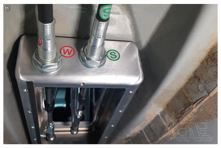
▶ Tighten the M16 nuts and make sure that there is no tension on the cables. Do NOT glue the nuts! (Picture 11)
