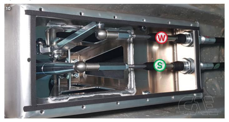
▶ The shift cables should be attached to the box as shown here.
