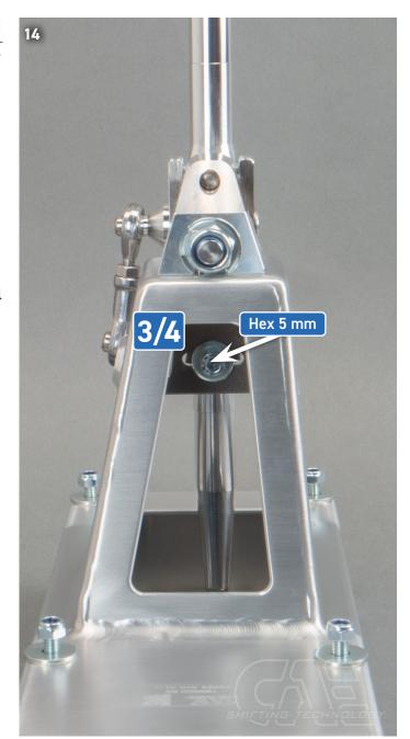
Screw cover plate under shifter box and again seal with foam rubber strip, glue screws in place, reinstall heat plates, exhaust, underbody trim, battery tray and battery and air filter.
