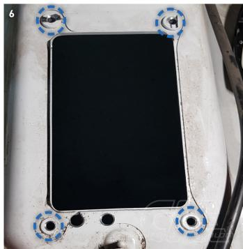
▶ Stick foam rubber strips on the shifter to ensure gas tightness during assembly, make sure that all holes in the base plate are covered. (Picture 7)
