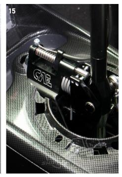
Screw cover plate under shifter box and again seal with foam rubber strip, glue screws in place, reinstall heat plates, exhaust, underbody trim, battery tray and battery and air filter.
