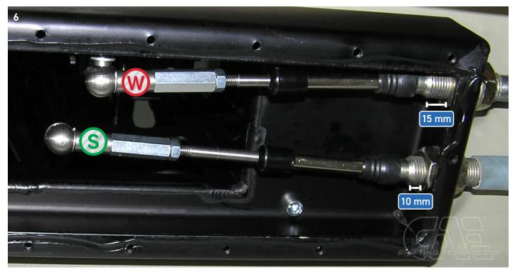
The shift cables should be attached to the box as shown here. Immediately route ropes toward engine compartment above transmission when installing. Tighten the M16 nuts until the pulleys are on block. !! DO NOT GLUE !!!
