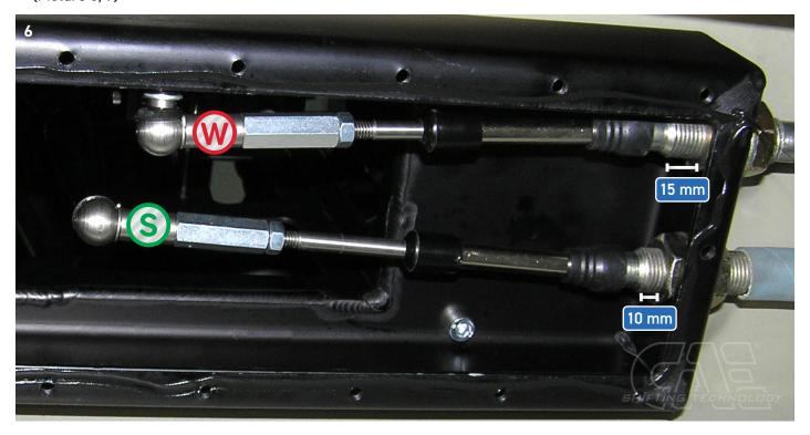
▶ The shift cables should be attached to the box as shown here. Immediately route ropes toward engine compartment above transmission when installing. Tighten the M16 nuts until the pulleys are on block. !! DO NOT GLUE !!!
