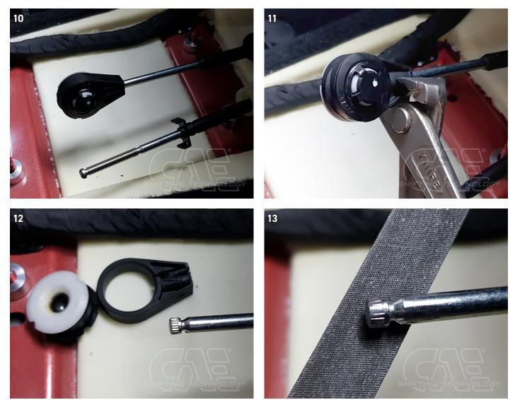
> The core of the selector cable (GASSE) must be shortened as shown in (Picture 14).
