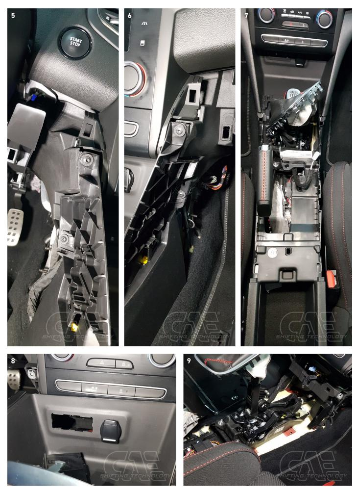
Remove the shift cables from the original gearshift bracket and loosen the 4 nuts. Remove the gearshift bracket.
