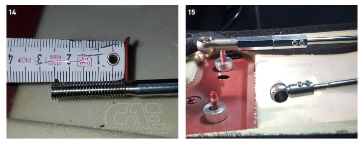
Slide the CAE cable ends/ball cups onto the machined cable cores and align them. (Picture 15) Tighten the grub screws with a 2.5 mm Allen key.
