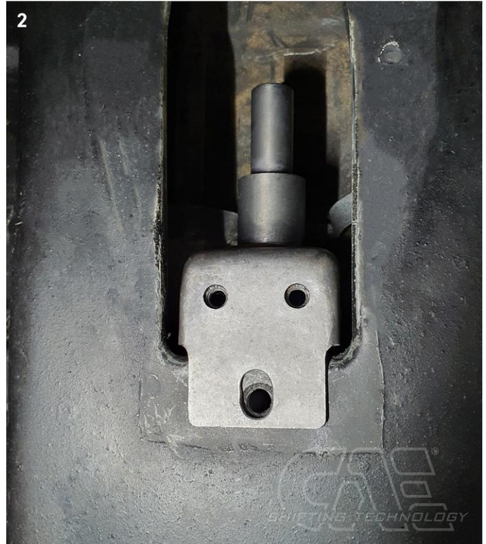
**i** For the shifter to function properly, it is absolutely necessary that the rear shift rod joint and the front bearing of the shift rod are free of play. It is essential to check this and replace the corresponding parts if necessary. The shift rod clamp at the rear joint of the shift rod should be adjusted to the shortest length. (Picture 2a)
