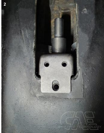
i For the shifter to function properly, it is absolutely necessary that the rear shift rod joint and the front bearing of the shift rod are free of any movement.
