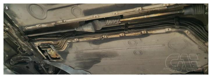
▶ Remove front support and shift rod linkage. (6-kt SW13) (Picture 7, 8)
