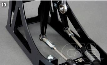
Press the greased ball cups onto the ball heads of the shift and selector levers.
