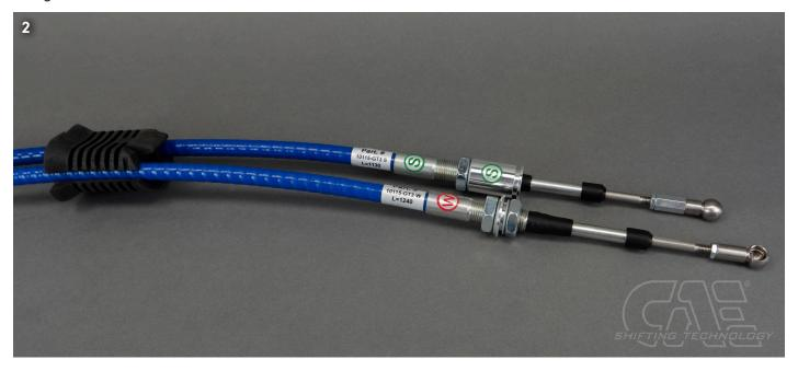
The length of the cables is preset, do not unscrew the aluminum adapters on the gearbox side!
