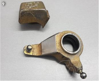
Reassemble the cable holder and the bell crank on the gear unit. (Picture 10) Grease the bearing of the bell crank well.
