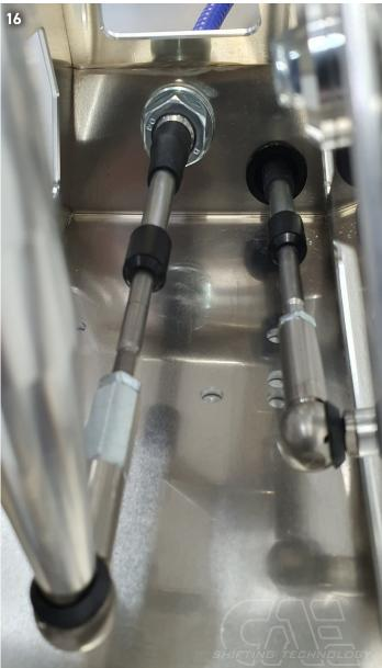
(i) PLEASE NOTE: ! Check cables for "end position free travel". When a gear is engaged, there must still be a residual travel available on the cable! (Picture A, B, C)
