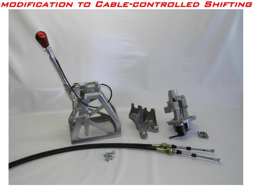
If center console is mounted, it must be dismounted or modified to achieve an acceptable space for the cables. The new unit should be mounted directly on to the floorboard, so part of the carpet must be removed.
