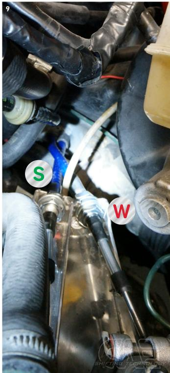
► Fasten the shift cables to the gearbox holder.
