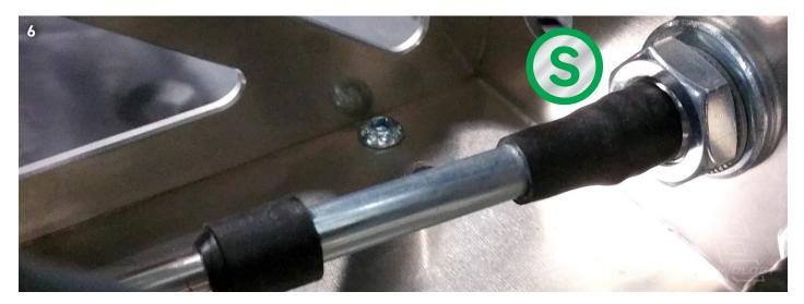
> Then screw on the ball heads and press them onto the shift lever.
