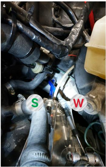
Fasten the shift cables to the gearbox holder.
