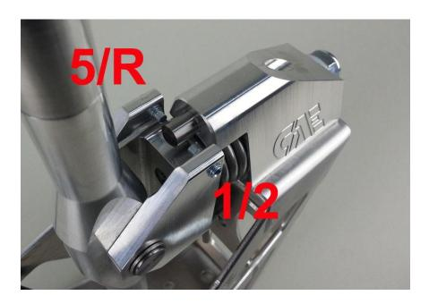
Select 1st / 2nd gear by lever and turn the right stopscrew till the gear 1 & 2 can be selected well.
