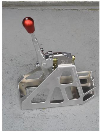
The shifter is intended for racing cars without interior equipment. If center console is mounted, it must be dismounted or modified to achieve an acceptable space for the shifter.
