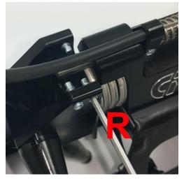
If the lower part of the lever collide with the right cable you should adjust the central position of the shift lever slightly more to the right, and start with step 1.
