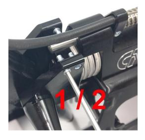
Pull the reverse mechanism at the Lever and select reverse gear. Screw in stop screw until the reverse gear goes in clean
