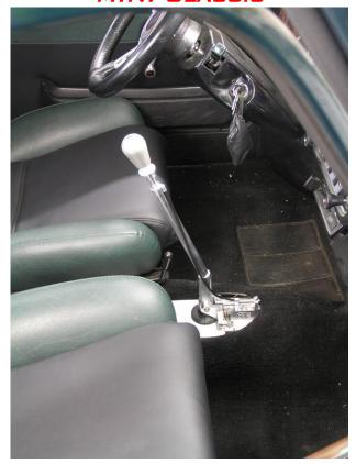
If center console is mounted, it must be dismounted or modified to achieve an acceptable space for the cables. The new unit should be mounted directly on to the floorboard, so part of the carpet must be removed.
