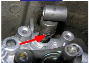
Replace the bolt from sleeve thru the delivered; it makes the sleeve asolutely free from backlash
