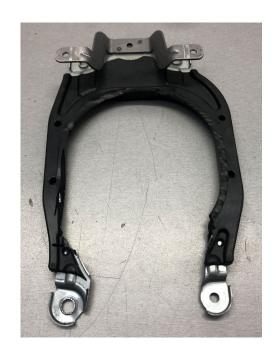
Now mount the frame over the sleeve. Make sure that the lower sleeve sits properly. The frame must press the sleeve firmly onto the transmission tunnel to make it tight.
