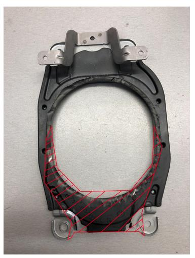
• Then cut out the frame in the red marked area.
