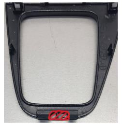
If the shift bag is desired, then the mounting frame must be cutted a little. (see marked area)  The center console must be cutted in the area of the power window switch. It must be made a hole in the power window switch for the reverse gear locking pin. (red marked area)
