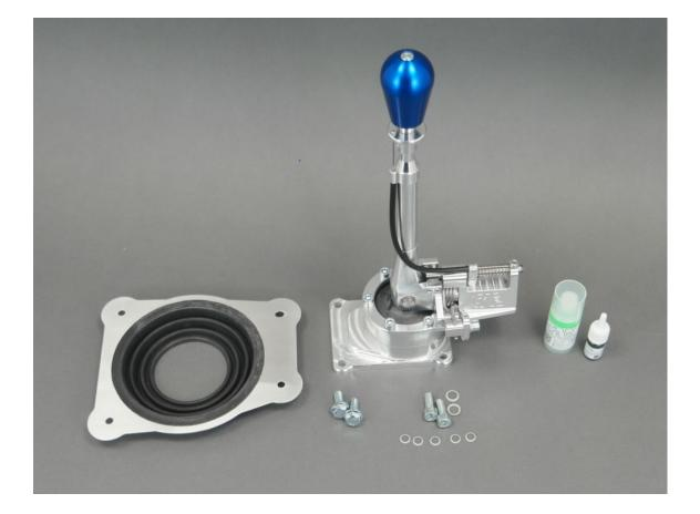
The shifter is intended for vehicles with interior fittings. The center console has to be slightly trimmed for installation until a freely moving for the shifter is guaranteed.
