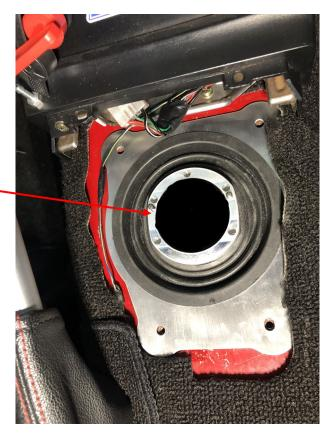
• Lubricate the lower ball of the gear lever lower part with a little gear oil and place the upper part of the gearbox from above. Hold the gearshift vertically and carefully insert the ball into the gearbox.
